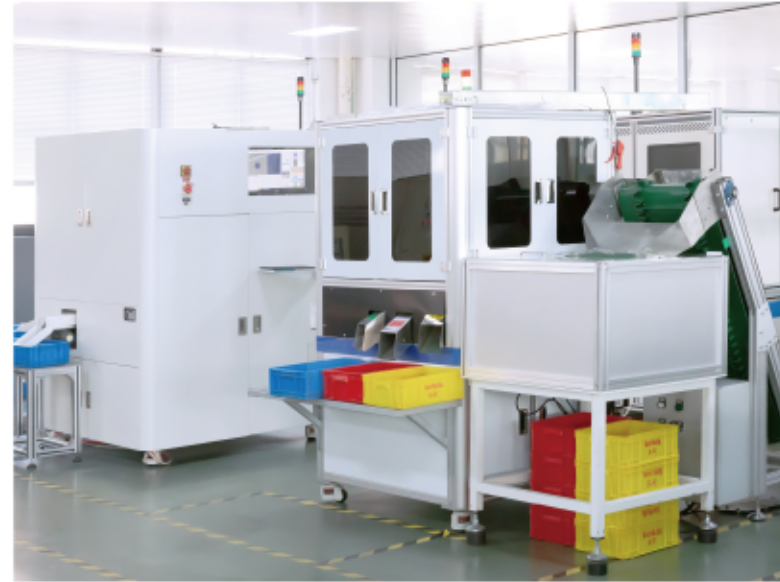
▲ 工业CCD外观检测仪 Automatic appearance and tolerance test instrument 对产品尺寸及外观进行全检 Automatically full inspection of product appearance and tolerance
